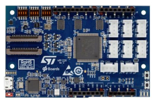
Figure 4.5: View of the central board Mezzanine B-F446E-96B01A. Adopted form [43].
