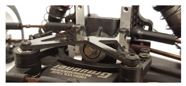
Figure 3.3: Detail of the front differential.
